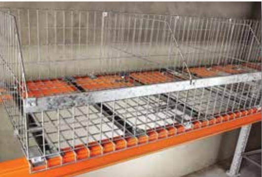
Mesh binning for small parts storage.
